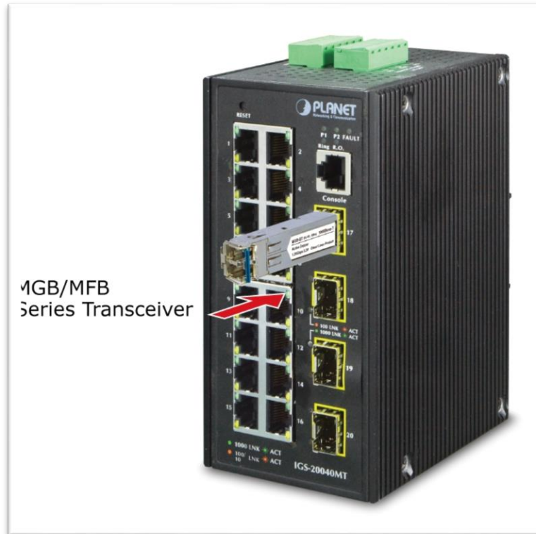
Figure 2-2: Plugging in the SFP Transceiver
